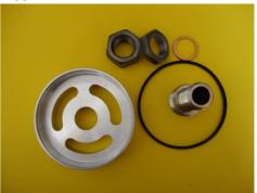
Ensure that the area around the oil filter housing is clean and remove the existing filter bowl. If fitted, remove the splash plate (this looks like a large steel washer) in the centre of the filter head. If there is a felt washer under the plate remove this also. Place a tommy bar through the hole in the anchor screw boss (the part into which the long filter-retaining bolt screws) and remove the boss.
